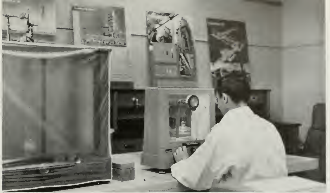
Weighing lucite-encased oil-producing rock was part of the process involved in the study of the effect of fluidity on the production of petroleum. These studies also pertained to soils and water-bearing formations. The oil industry closely follows the work done in this part of the department.
